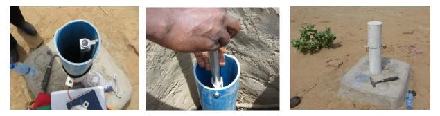
A data logger hunging inside the borehole by means of a ring. Installation of a data logger inside the borehole
